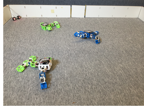
(d) Scheme D: Embodied evolution of controllers and bodies. There is no centralized evolution manager, selection and reproduction are regulated by the robots and their interactions.
